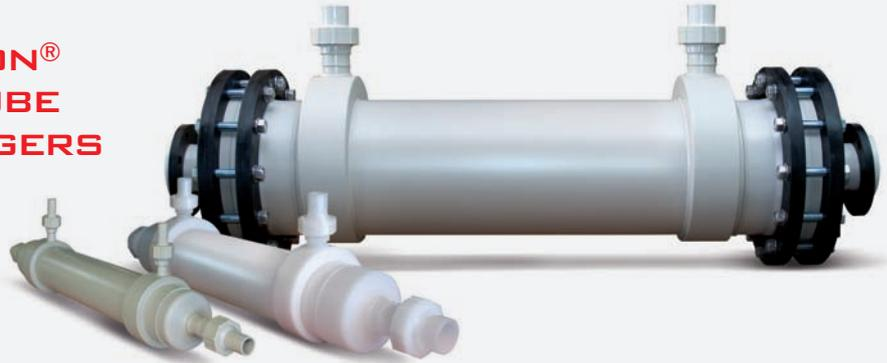
Shell and tube heat exchangers consist of an external shell tube and internal multiple hoses which consist of a large number of hoses of small nominal diameter. The internal hoses are welded in two perforated bases, which are then welded to the external shell tube. The first medium flows through the external shell tube and the second medium flows through inside the hoses. The hotter medium is cooled down and the cooler medium is heated up in this operation.
