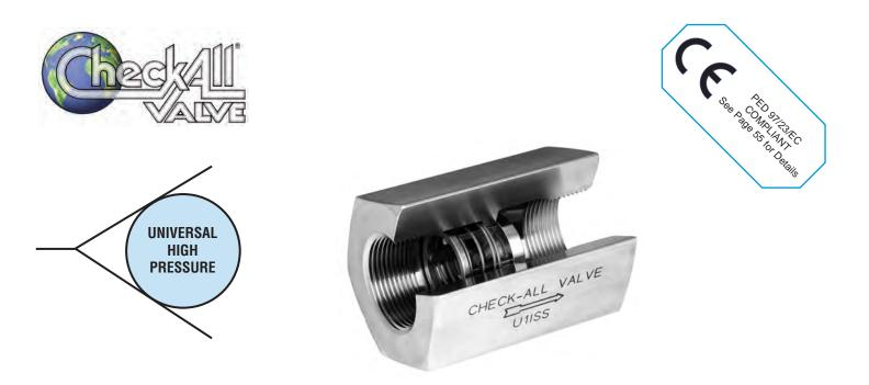
The **Universal High Pressure (U1, R1)** check valve is a one piece body machined from bar stock with female pipe threads. The valve is designed and manufactured for high pressure applications. These valves can also be used as low pressure relief valves or vacuum breakers by using the desired spring settings. This valve is normally supplied with a "metal-to-metal" seat. NPT threads are per ASME B1.20.1. Also available with ISO 7 "Rp" threads. (R1).
