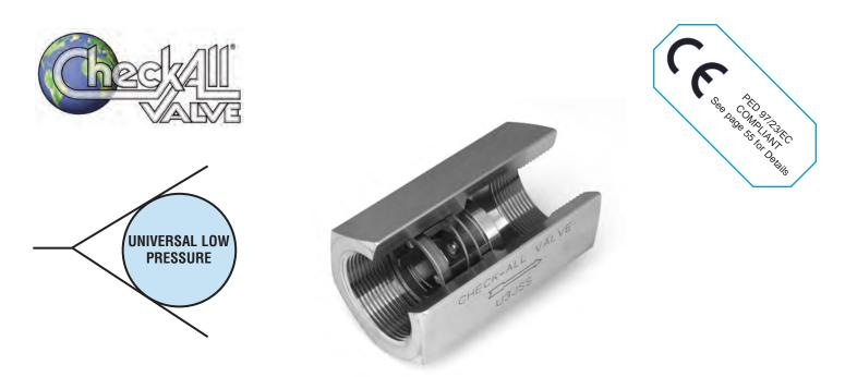
The **Universal Low Pressure (U3, UR)** check valve is a one piece body machined from bar stock and is designed for minimum pressure drop. The valve has a light-weight, compact design that provides maintenance-free, dependable service. NPT threads are per ASME B1.20.1. Also available with ISO 7 "Rp" threads. (UR). These valves can also be used as a low pressure relief valve or vacuum breaker by using the desired spring settings.
