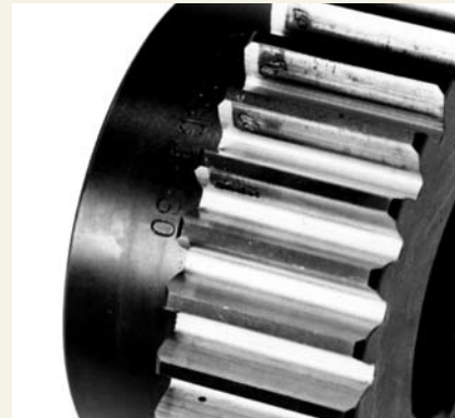
Poor tooth contact and pitting
