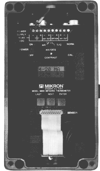
Temperature transmitter — Alphanumeric LCD (8 characters x 2 lines) displays temperature and output type. Enclosure of temperature transmitter of M668 meets NEMA 1 through 13 requirements.
