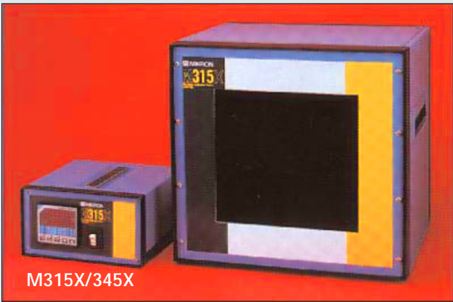
Large area low temperature blackbody source.
