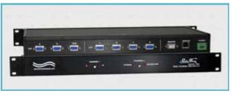
CROSSOVER position is defined as port A connected to port D and port B connected to port C. Remote Control access can be accomplished using an Ethernet 10/100BASE-T connection and either Telnet commands or graphical user interface. The unit can also be controlled via RS232 ASCII commands through the rear panel DB9 Remote Port.
