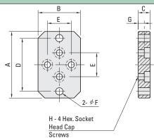
For use with the standard swing clamps shown above. These plates attach to the swing clamps and allow for easy fastening and top side mounting. Made from SAE-1045 alloy steel with black oxide finish.
