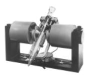
Determine magnetic separation characteristics of ores and check plant concentrate and tailing quality.
