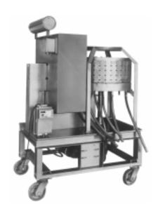
High intensity wet magnetic separators for the separation of weakly magnetic materials.
