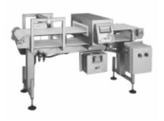
Eriez lab conveyors are a modular design that will accept metal detectors with a range of aperture heights and widths to accommodate the range of customer product samples. Several types of reject devices are available on the lab conveyors, including variable speed drives to adjust product speeds to match the customer requirements.
